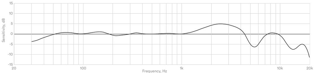
Note: Frequency response is measured with attached foam cap
